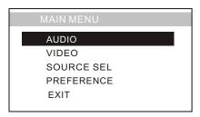
The main menu includes 5 selections above, press ▲or ▼ button to select the requisite item, then hit ENTER to set it; press ▲or ▼ button to reach EXIT, press ENTER to exit setting.
